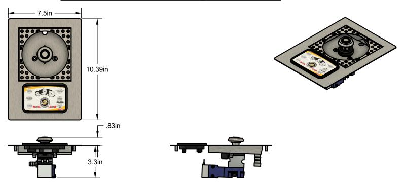
Dispenser needs a minimum clearance of 3.5" from top of counter to bottom of valve bodies. Underside of dispenser must be accessible for service work. Dispenser requires a standard 120VAC outlet within 10 feet of location.
