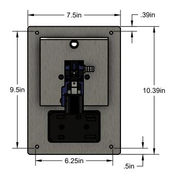
Minimum Cut Dimension is 6.25" X 9.5". DO NOT cut over 7.5" X 10.39".
