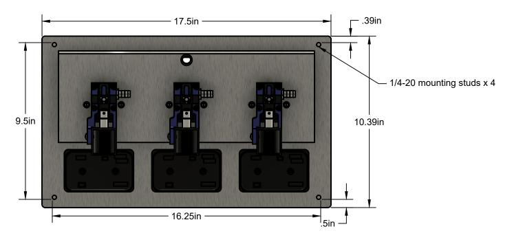
Minimum Cut Dimension is 16.25" X 9.5". DO NOT cut over 17.5" X 10.39".
