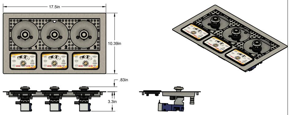
Dispenser needs a minimum clearance of 3.5" from top of counter to bottom of valve bodies. Underside of dispenser must be accessible for service work. Dispenser requires a standard 120VAC outlet within 10 feet of location.
