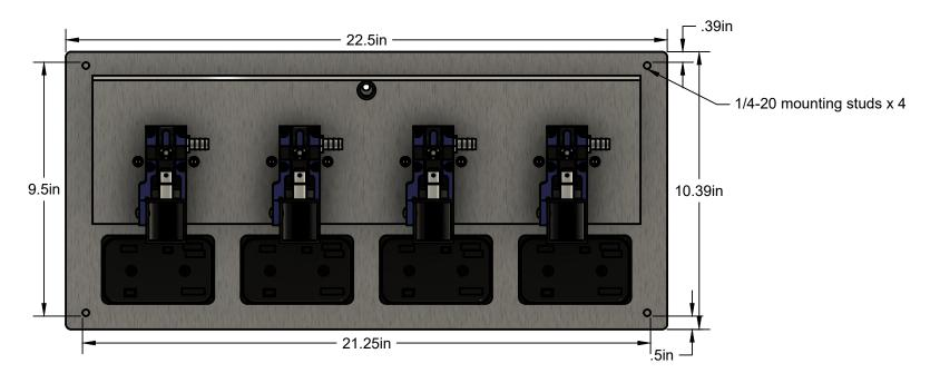
Minimum Cut Dimension is 21.25" X 9.5". DO NOT cut over 22.5" X 10.39".
