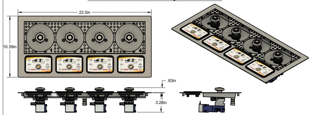
Dispenser needs a minimum clearance of 3.5" from top of counter to bottom of valve bodies. Underside of dispenser must be accessible for service work. Dispenser requires a standard 120VAC outlet within 10 feet of location.
