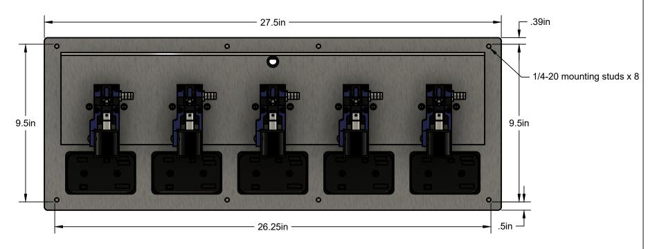
Minimum Cut Dimension is 26.25" X 9.25". DO NOT cut over 27.5" X 10.39".
